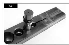
Fit tip and nut into holding tool and clamp tool into bench vice.
